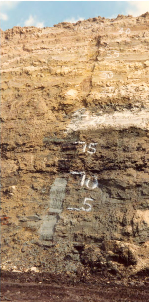
Figure 2 – Overburden profile in highwall and detail of redox boundary (numbers painted on highwall denote distance in feet above top of lignite seam)
