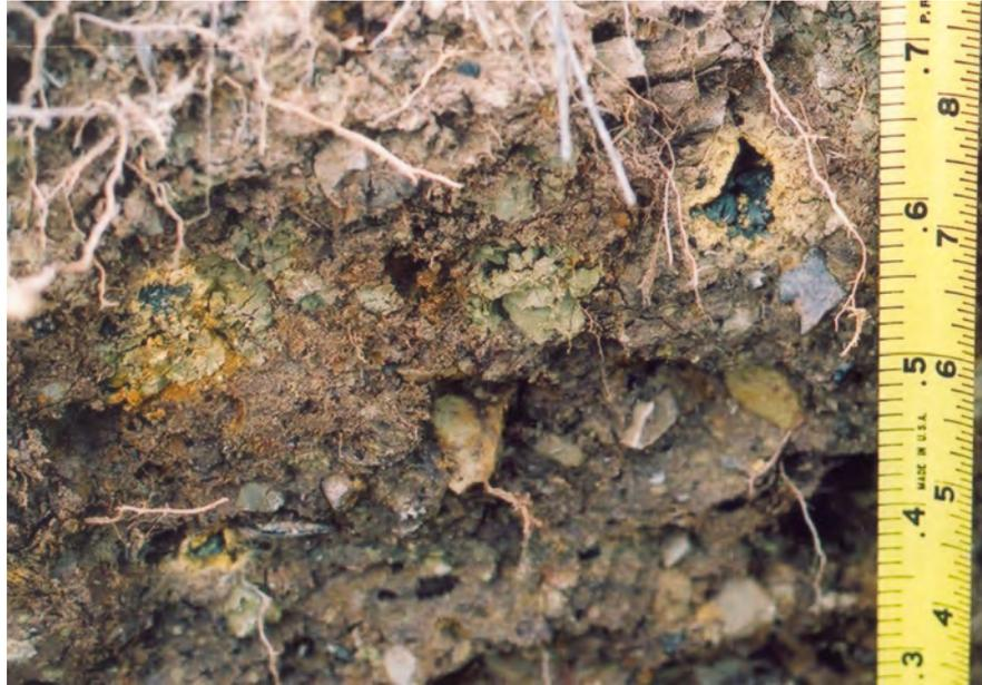
Figure 7 – weathered pyrite nodule with iron oxyhydroxide “rind”
