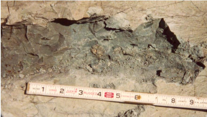
Figure 2 – elongated pyrite nodules *in situ* in paleosol in highwall (stereophoto)
