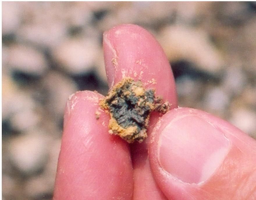
Figure 6 – pyrite nodules weathering *in situ* in minesoil
